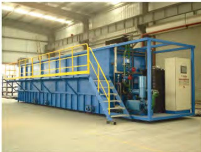
The modular concept allow for phased construction of wastewater treatment plants and makes it adaptable to a wide range of sizes and flow rates. COMPACT can be delivered as a containerized unit. This solution has important advantages such as:
